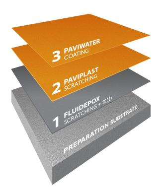
The final thickness of the resinous covering is around 2 mm.
